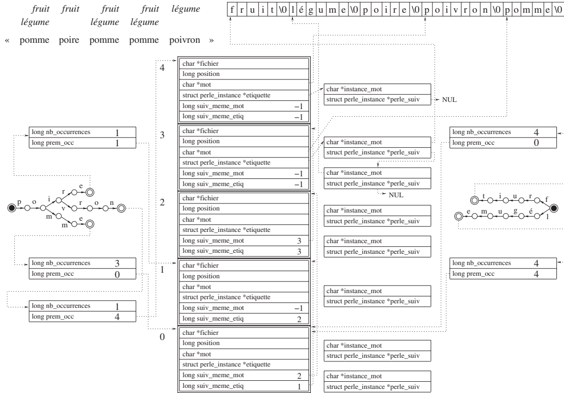
Fig. 4. The specialized index table format developed for this application. At the center, the table of token occurrences (used to compute matrix W by moving a contextual window). At the left, a trie (lexical tree) indexing the words of the vocabulary. The table may also be used for tagging, hence the use of the “etiquette” labels and of the second trie on the right (useful to index the tags of the tagset). The figure exemplifies the result of indexing a text containing the words “pomme poire pomme pomme poivron”.
